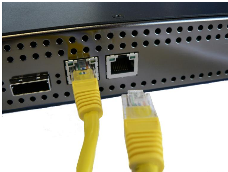
Front Panel of the Bridge Showing Ethernet Cable Connections
