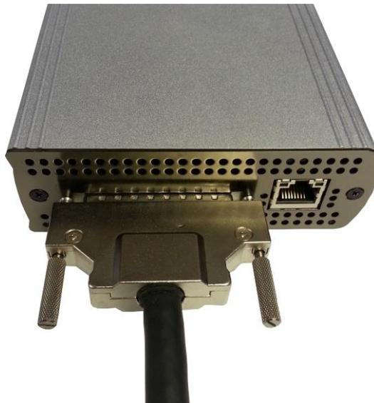
**Connecting the SCSI Cable to the Bridge SCSI Port**
