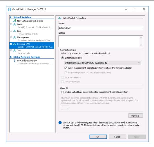
Ensure that the checkbox labeled *Allow management operating system to share this network adapter* beneath the physical network connection dropdown menu is checked.
