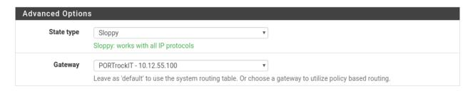
On WAN Link Gateway B, add a new firewall rule. This rule covers accelerated return traffic from the Destination Endpoint to the Source Endpoint. The following fields must be modified:
