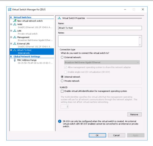
In the new properties section select a name for the network connection.
