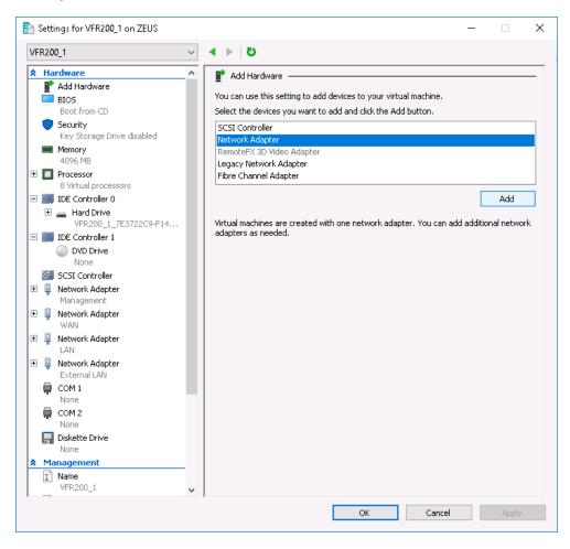
At this point an empty Virtual Switch is displayed. Choose the newly created internal switch from
