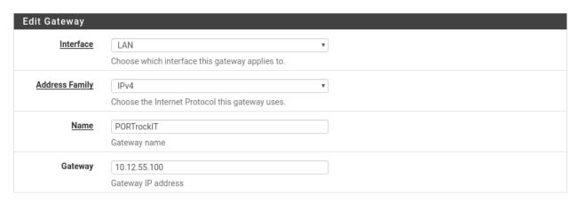
Similarly, on WAN Link Gateway B, the LAN IP address of PORTrockIT Node B must be added as a gateway.
