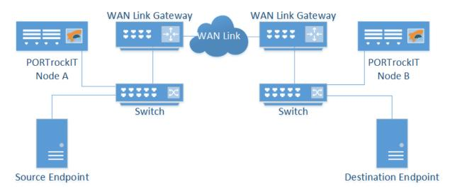
In this case data is accelerated from the *Source Endpoint* to the *Destination Endpoint*. *Node A* is set up to intercept traffic leaving the *Source Endpoint*, accelerating any data that matches the protocol across the *WAN Link* to the connected *Node B*. The traffic then continues on normally to its intended destination.
