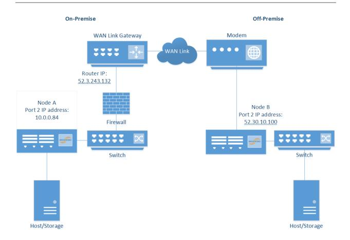
In this example the IP addresses for establishing a Nodal link are the IP address of the router connected to Node A, and the public IP address of Node B.
