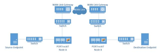
In this case data is accelerated from the *Source Endpoint* to the *Destination Endpoint*. *Node A* is set up to intercept traffic leaving the *Source Endpoint*, accelerating any data that matches the protocol across the *WAN Link* to the connected *Node B*. The traffic then continues on normally to its intended destination.
