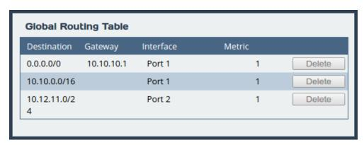
Currently *Node A* doesn't know how to reach the 10.12.12.0/24 network so traffic for the *Endpoint* will be lost. To resolve this, a static route needs to be added.
