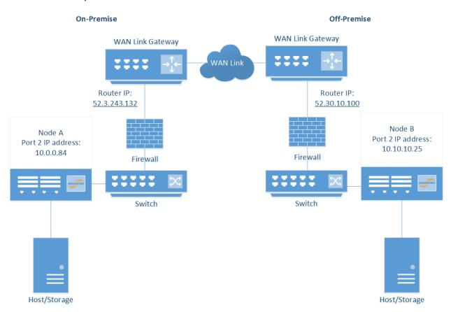
In this example the IP addresses for establishing a Nodal link are the IP addresses of the router, in this case:
