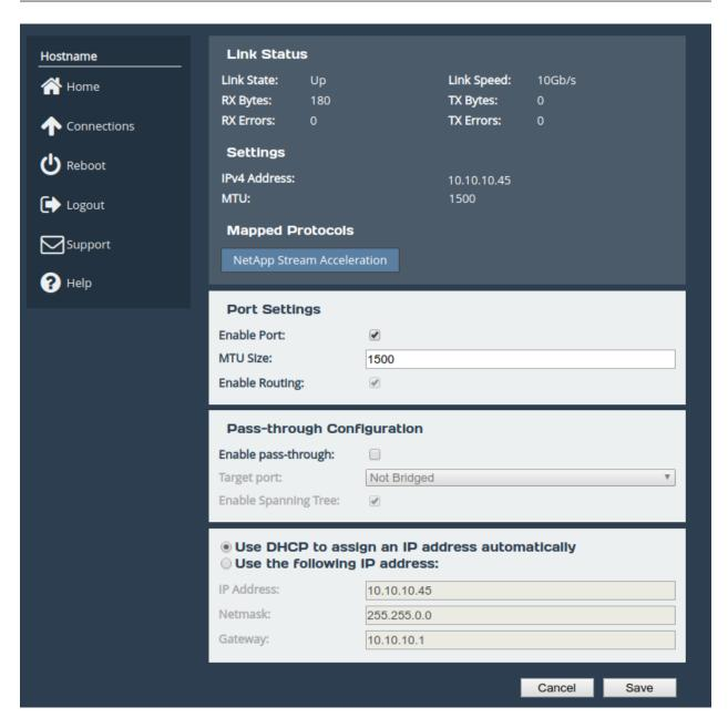
In the *Pass-through Configuration* section ensure *Enable pass-through* is checked and select the mapped WAN port as the *Target port*, by default this will be *Port 2* as shown below:
