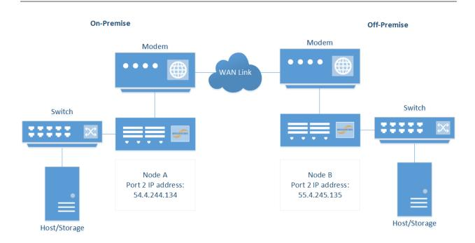
In this example the IP addresses for establishing a Nodal link are the public IP addresses assigned to *Port 2* on the Bridgeworks Nodes:
