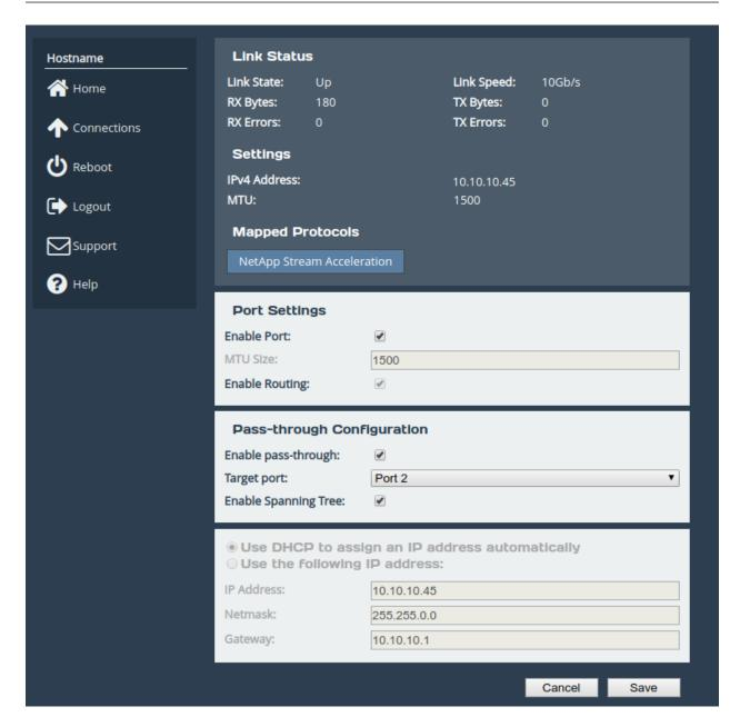
To protect against network issues, the PORTrockIT unit participates in STP (Spanning Tree Protocol) by default to ensure that network loops are not created. Note that PORTrockIT acceleration is disabled when a network loop is detected.
