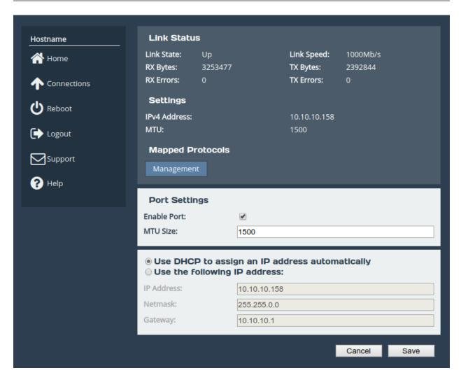
The port settings page allows the IP address of a port to be manually assigned. To do so, select the radio button *Use the following IP address*. The fields *IP Address*, *Netmask* and *Gateway* are now available to be filled in. When all fields are complete, click the *Save* button. A reboot is required for the changes to take effect.
