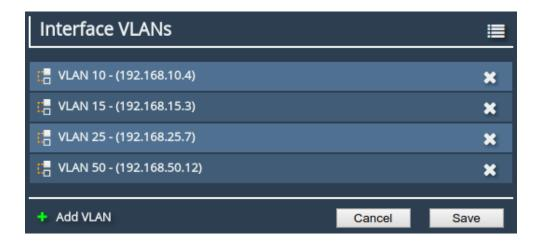
VLANs can be added to an interface by pressing the *Add VLAN* button. When the button is pressed an *Add VLAN* dialogue will appear. A VLAN can be created with an ID between 1 and 4094. A maximum of 64 different VLANs can be added to the PORTrockIT. To queue the VLAN for addition, press the *OK* button. The VLAN will not be added to the interface until the changes are committed. If the *Cancel* button is pressed or the page is navigated away from, the VLAN will not be added.
