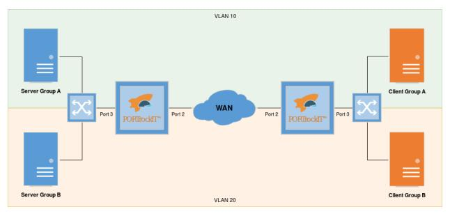
This guide assumes that there is an active connection between the two PORTrockIT Nodes in each local area network (LAN), with Port 2 and Port 3 set up in *Bridged In-Line* topology.
