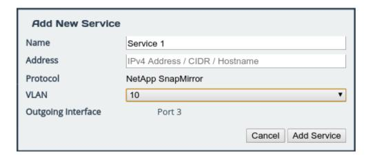
The VLANs dropdown field allows for a single VLAN to be chosen for each service. This way, even with the same address and interface data being used, accelerated traffic can be selected by VLAN.
