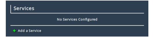
To add a service, click on the *Add a Service* button. This will show a dialog box where local server details can be added. The *Name* field can be changed to something more descriptive if desired. Add the address of the local service into the *Address* field. Options for the address are IPv4, CIDR or a resolvable DNS address.
