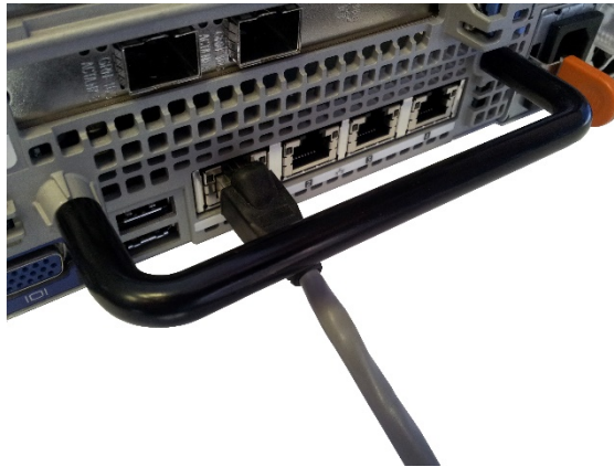
Rear Panel of the Appliance Showing Ethernet Cable Connections
