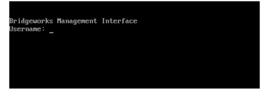
To reset the password of a user account using the SSH method, connect to the Gateway via SSH to access the login prompt.
