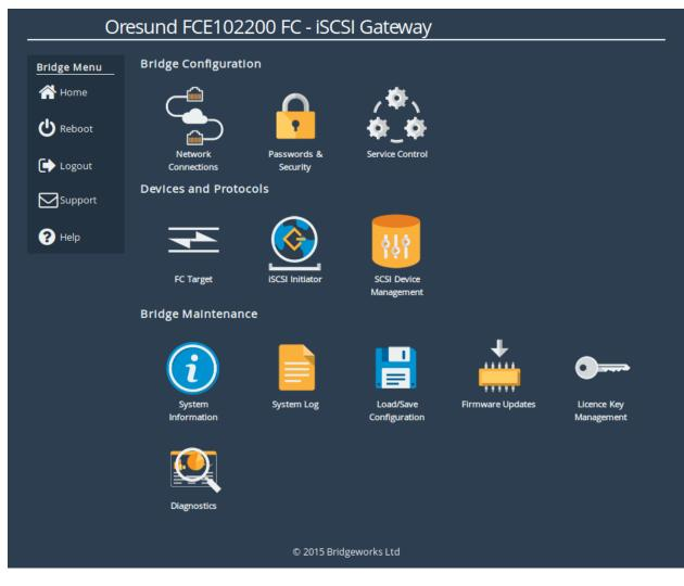
The web interface is split into two sections. The left hand *Bridge Menu* panel typically remains constant wherever you are within the web interface. It allows you to reboot or logout of the web interface. The Home link may be used from any page to return to the Home screen.
