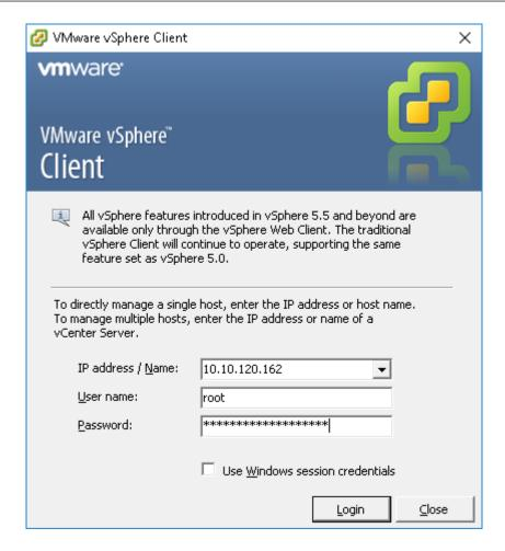
Enter the IP address or server name of the target ESXi host. If applicable, fill out the username and password and click login.
