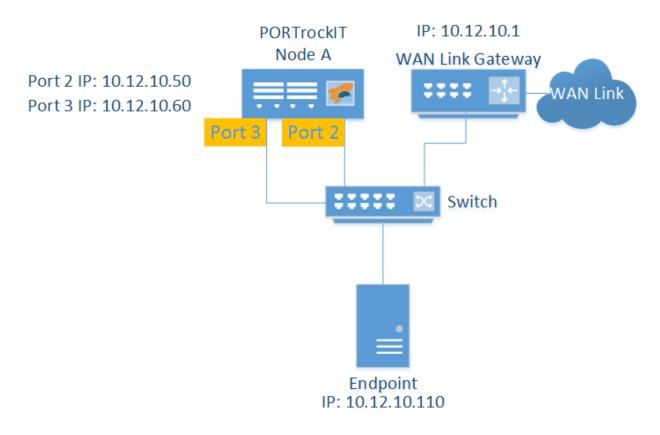
This example explains the routing needed on *Node A*, which has the following 3 ports:
