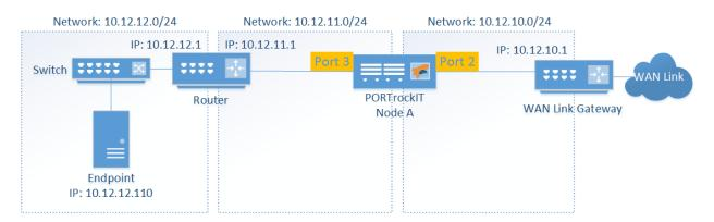
This example explains the routing needed on *Node A*, which has the following 3 ports:
