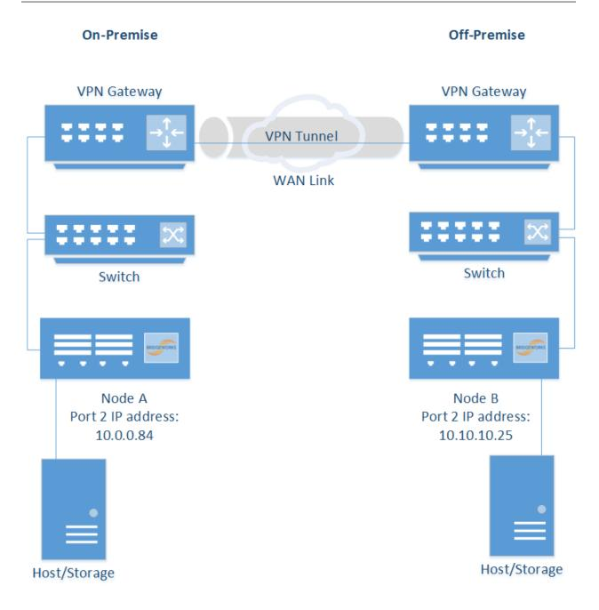
In this example the IP addresses for establishing a Nodal link are the private IP addresses assigned to *Port 2* on the Bridgeworks Nodes:
