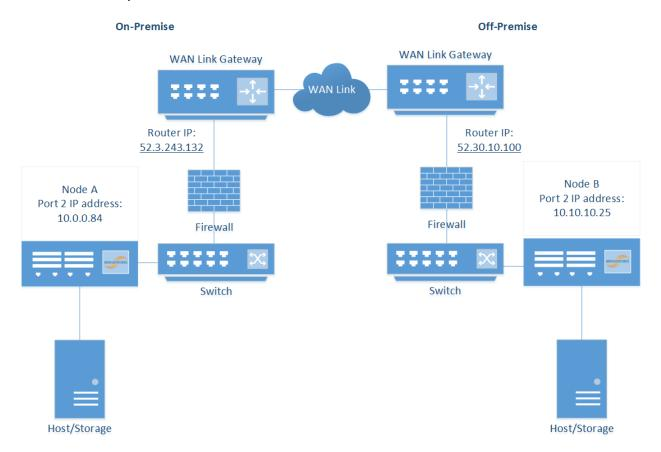
In this example the IP addresses for establishing a Nodal link are the IP addresses of the router, in this case:
