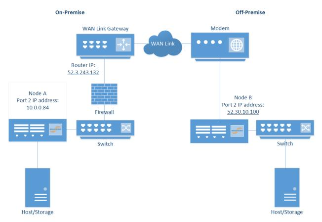
In this example the IP addresses for establishing a Nodal link are the IP address of the router connected to Node A, and the public IP address of Node B.
