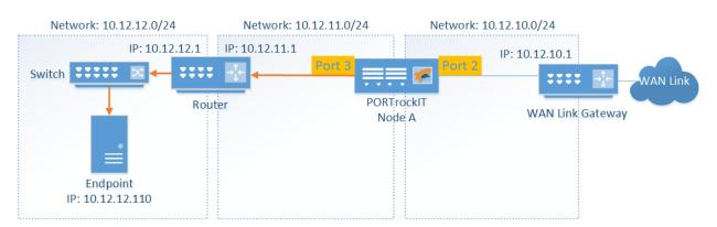
Network traffic for the *Endpoint* will be sent from *Port* 3 and be directed through the router.
