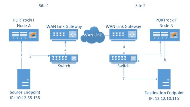
In this topology *Node A* is in the "Bridged Physically-In-Path" mode of operation and *Node B* is in the "Out-of-Path" mode of operation. The "Out-of-Path" mode can only be used when you are looking to accelerate traffic in a client/server relationship, such as object storage or FTP, and can only be used on the server site.
