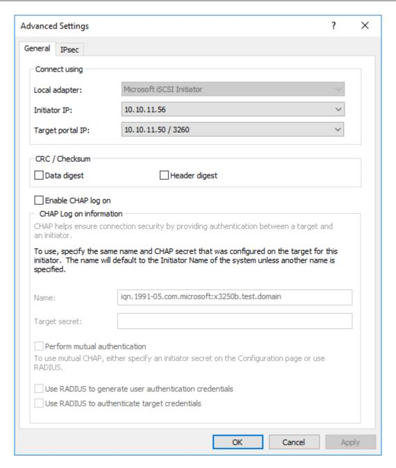
In the *Connect using* section, select the *Initiator IP* address and the *Target portal IP* address for the new connection. In most instances these should be different from the source and target addresses of the original connection. In this example we have connected to 10.10.10.50 / 3260 as the leading connection, and the second connection will be 10.10.11.50 / 3260.
