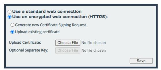
If you simply click *Save* without uploading any files for the certificate or key, a self-signed certificate will be automatically generated by the Gateway.
