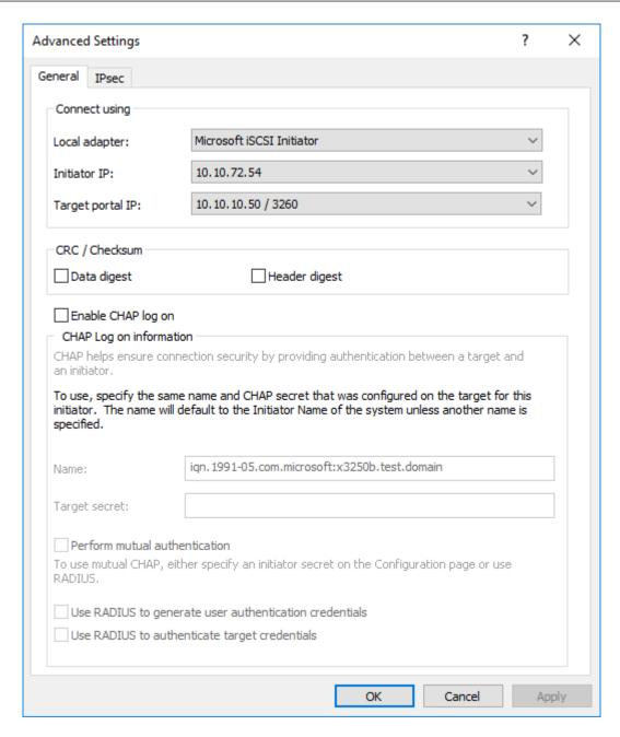
The Advanced Settings page is the same as that of the discovery except for one addition. In the *Connect using* section, there is a *Target portal IP* option. This allows you to choose which interface of the iSCSI Gateway will be used to make the connection to the target. In this example we have chosen to connect to the IP address 10.10.50 on port 3260.
