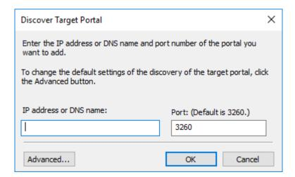
Enter the IP address for the iSCSI Target. In this example we shall use the IP address 10.10.50.
