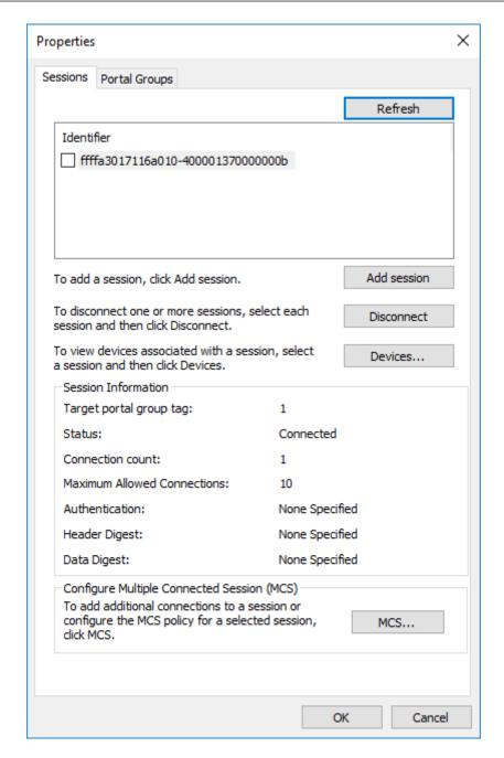
In this window you can view the iSCSI Sessions associated to the iSCSI Target, how many connections are attached to each iSCSI Session, and the Target Portal Group.
