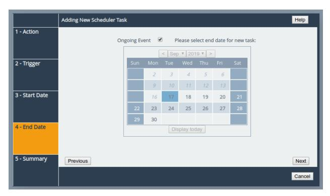
On the End Date section of the wizard, you can pick the end date for the new task. You can either select the *Ongoing Event* checkbox for a task that should run until cancelled, or select a date using the calendar. The selected date will be marked with a red cross.
