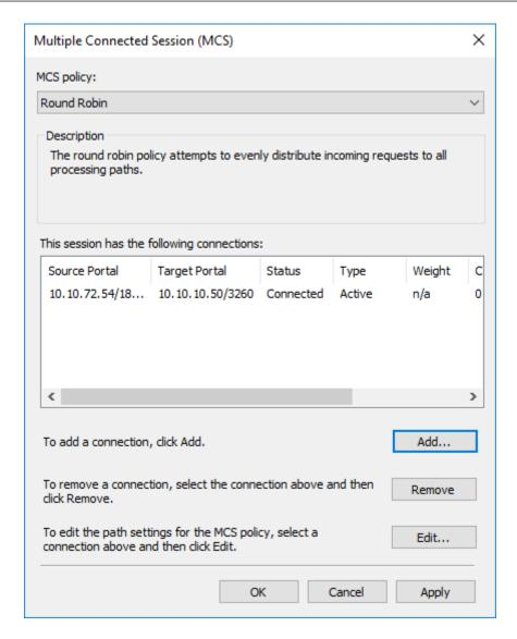
This shows how many iSCSI Connections are active and the type of load balance used. For all iSCSI Sessions, there will be at least one leading connection.
