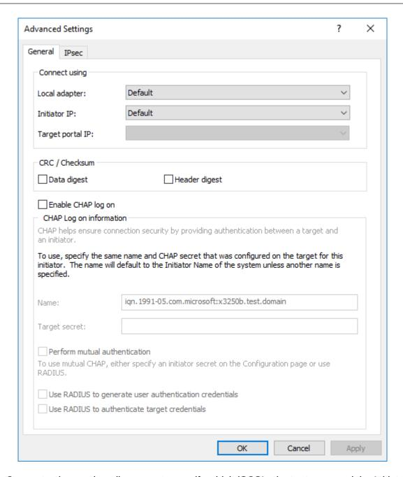
The *Connect using* section allows you to specify which iSCSI adapter to use and the Initiator IP. The *Local adapter* should only differ from Microsoft iSCSI Initiator if an iSCSI offload card has been installed. For the purpose of this guide, we shall only use the Microsoft iSCSI Initiator. Leaving this setting as *Default* will also use the Microsoft iSCSI Initiator.
