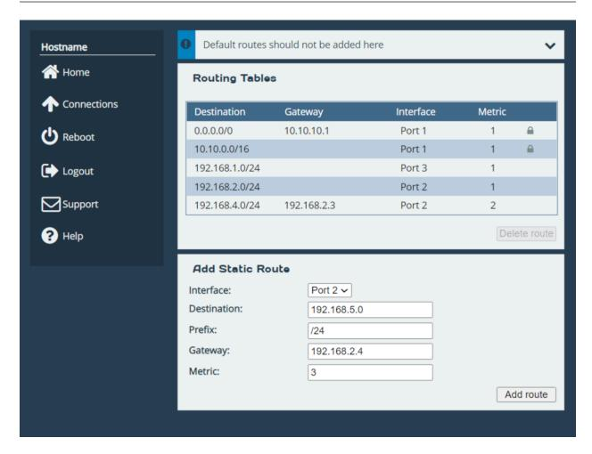
In this example, a route is being added to 192.168.5.0/24 via the gateway at 192.168.2.4 on Port 2. The route has a metric of 3.
