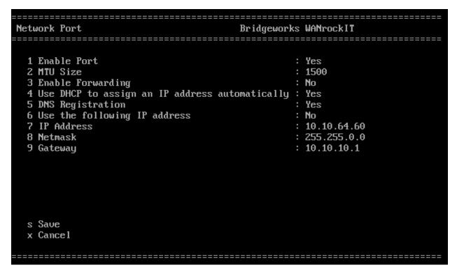
Ensure this port is enabled by checking the Enable Port option. If this says No next to it, select it,
