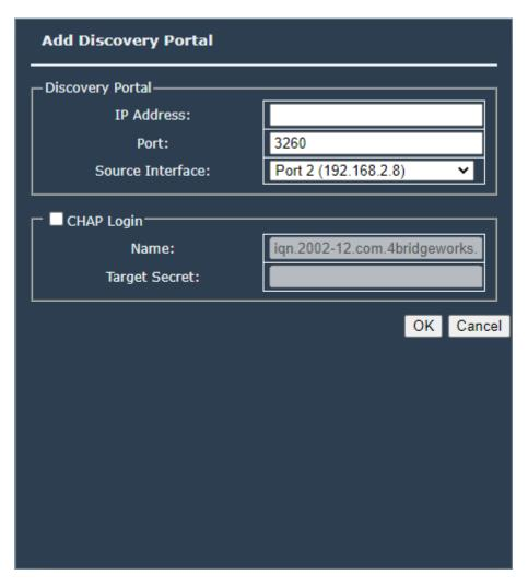
Insert the *IP Address* of the iSCSI target portal you wish to connect to and select the *Source Interface* from the drop down list.
