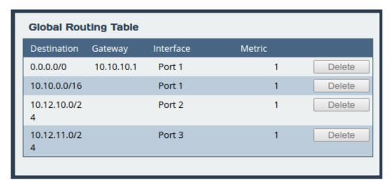
Currently *Node A* doesn't know how to reach the 10.12.12.0/24 network so traffic for the *Endpoint* will be lost. To resolve this, a static route needs to be added.
