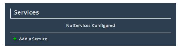
To add a service, click on the *Add a Service* button. This will show a dialog box where local server details can be added. The *Name* field can be changed to something more descriptive if desired. Add the address of the local service into the *Address* field. Options for the address are IPv4, CIDR or a resolvable DNS address. Then select the *Out of Path* checkbox.
