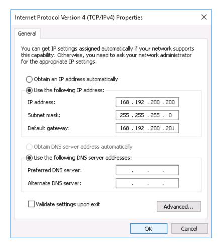
Enter the IP address and subnet mask to allow it to communicate with the settings that are used for the same Virtual Switch on the PORTrockIT.
