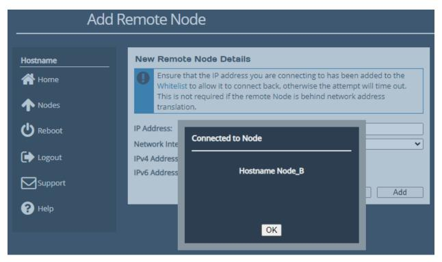
The next stage is to perform Node discovery in the other direction. From the *Node Management* of Node B, click the *Add Node* button to bring up a dialog box, and enter the IP address of the WAN port of Node A. Click *Add* to negotiate a connection between the Nodes.
