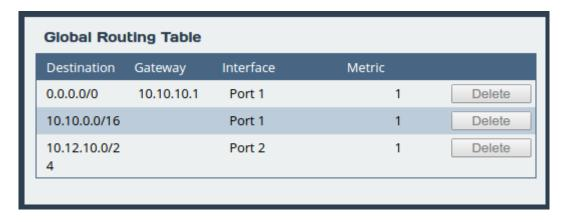
Currently *Node A* will be sending traffic destined for the *Endpoint* from *Port 2* instead of *Port 3*. To resolve this, a static route needs to be added.
