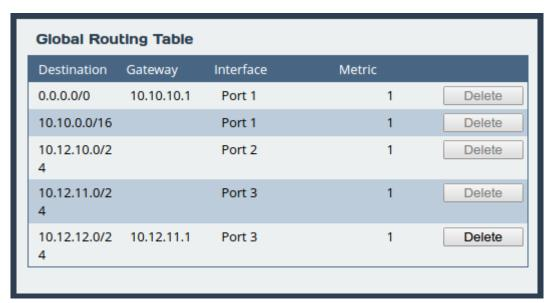
Network traffic for the *Endpoint* will be sent from *Port 3* and be directed through the router.
