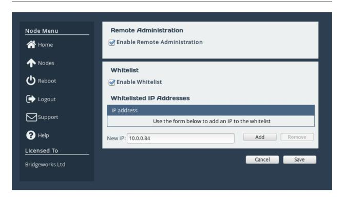
When this has been added successfully you will see the IP address entry added to the list, as shown below.
