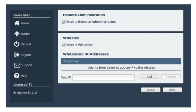
Under *New IP*, enter the IP address of the WAN port of Node A in the entry box, and click the *Add* button.
