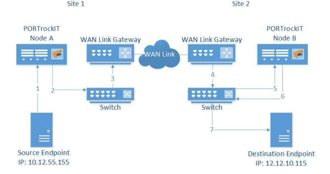
In this topology *Node A* is in the "Bridged Physically-In-Path" mode of operation and *Node B* is in the "Out-of-Path" mode of operation. The "Out-of-Path" mode can only be used when you are looking to accelerate traffic in a client/server relationship, such as object storage or FTP, and can only be used on the server site.
