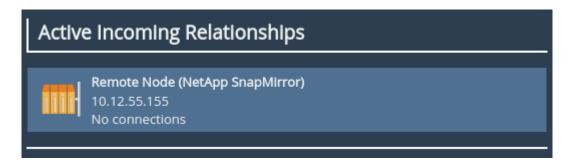
If the relationship is displayed in the *Active Incoming Relationships* list then the relationship was successfully created. After this, the software configuration required for accelerating traffic between PORTrockITs is complete.
