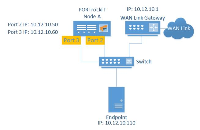
This example explains the routing needed on *Node A*, which has the following 3 ports:
