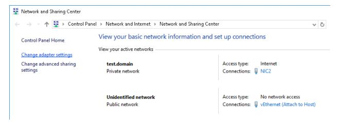
In the *Network Connections* window there will be a vEthernet with the same name given in the *Virtual Switch Manager*.
