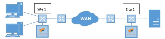
This mode can be considered an extension of the "Logical-In-Path" mode, where the PORTrockIT communicates with the L3 switch or router that is implementing the routing policies. This communication allows the router to ensure the PORTrockIT is operational prior to sending traffic to be accelerated, and allows automatic load-distribution for PORTrockIT units with multiple LAN ports.
