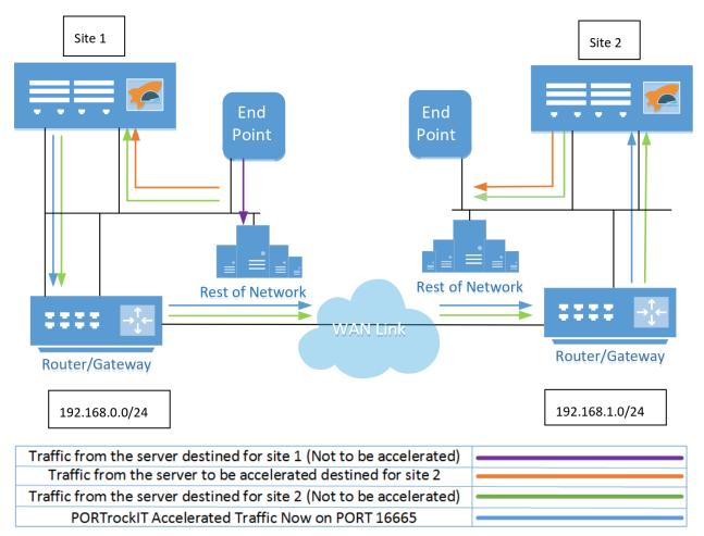
If routing policies are not specific on the server, all traffic destined for "Site 1" can be routed to the PORTrockIT Node which will forward the traffic to "Site 1"'s primary router (Green arrows). For example: The IP address of the LAN port of the PORTrockIT Node at "Site 1" is set to "192.168.0.10". The following policy routing rule is added to the server at "Site 1".
