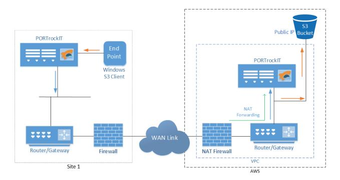
In this example, "Site 1" is configured to be in "Bridged-In-Path", in "AWS" the PORTrockIT Node is configured to be in "Out-of-Path" mode and is deployed as an EC2 image. The object store and the PORTrockIT are not in the same network domain and the object store is an externally hosted service preventing its routing from being modified.
