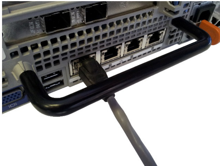
Rear Panel of the Appliance Showing Ethernet Cable Connections
