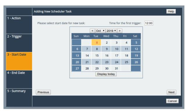
On the Start Date section of the wizard, you can pick the starting date and time for the new task. Enter a time into the *Time for the first trigger* box and select your start date using the calendar. The selected date will be marked with a red cross.
