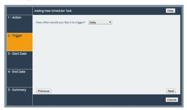
On the Trigger section of the wizard, you can pick the frequency of the event. The options are:
