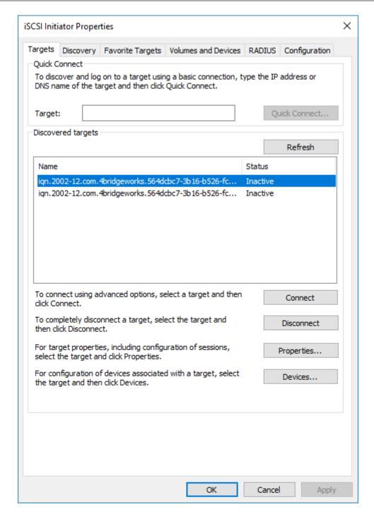
In this example two iSCSI targets have been discovered. The first device is the tape drive, and the second is the media changer. If no devices are displayed, check that the settings used to perform the discovery, including CHAP settings, are correct. Then return to *Targets* tab and click *Refresh*.
