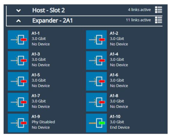
The name of an expander signifies its origin, and its level. For example, an expander named **2A1** originates from the  $2^{nd}$  host, from physical port **A**, and is the  $1^{st}$  level of expander from that port.
