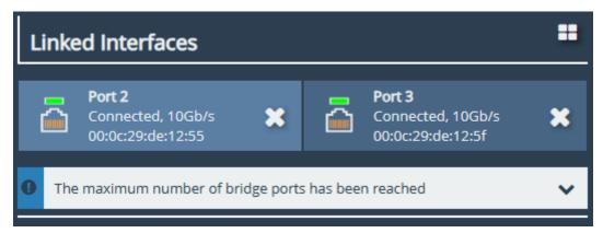
Please ensure these Nodes are not connected to the same Ethernet segment. To help protect against network issues, the PORTrockIT unit participates in STP (Spanning Tree Protocol) by default to ensure that network loops are not created. However this will prevent the PORTrockIT unit from operating as an acceleration device if it has to disable its bridging to protect the network.
