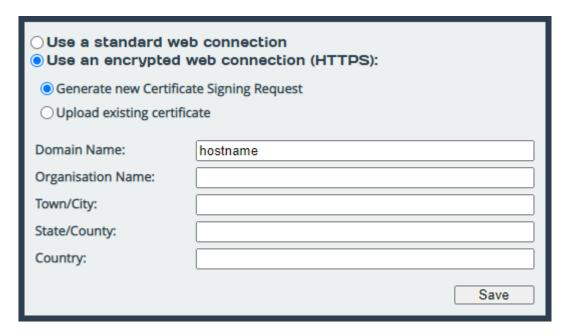
If you need a certificate signed by an external certificate authority, you may use the *Generate new Certificate Signing Request* option to do so. Select *Use an encrypted web connection (HTTPS)*, then *Generate new Certificate Signing Request* to open the form.
