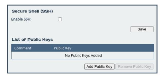
To enable SSH on network interfaces with the "Management" protocol mapped, tick the *Enable SSH* checkbox and click *Save*.
