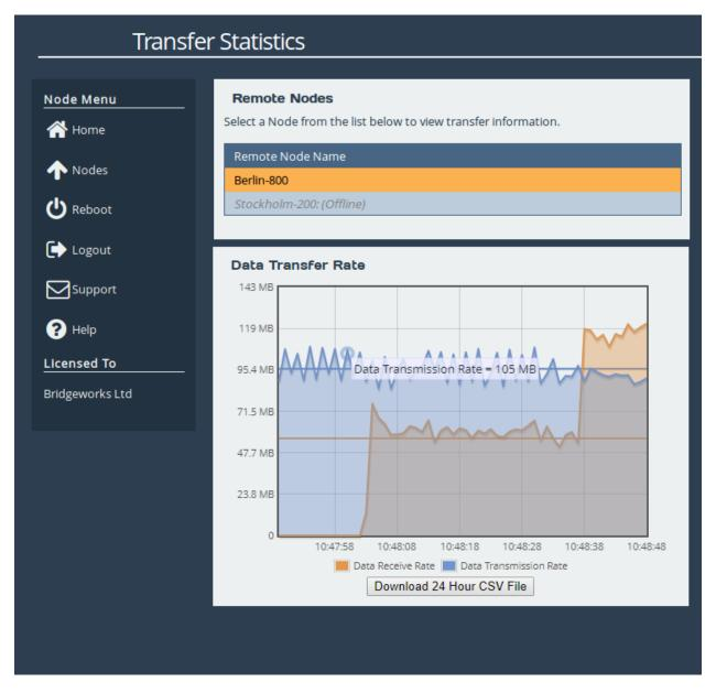
To view a remote Node's transfer rate, click on the name of the Node from the *Remote Node Name* list, and graphing will start automatically.
