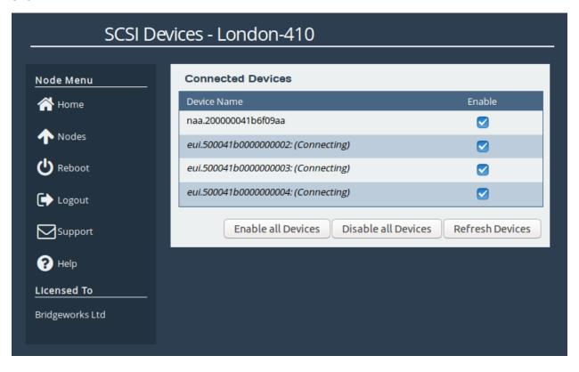
All the functionality that can be used when a Node is active can be used whilst a Node is connecting but the effects will not occur until the link is up.
