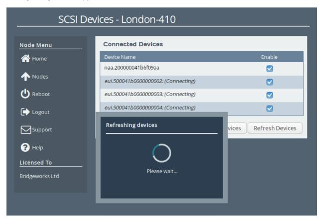
Once the refresh process has completed, a dialog box will appear to notify you about the connected Node and attached devices, as shown:
