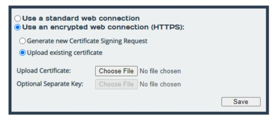
If you simply click *Save* without uploading any files for the certificate or key, a self-signed certificate will be automatically generated by the Node.
