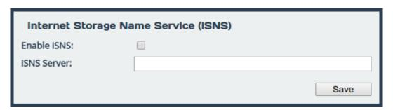
Internet Storage Name Service allows automated discovery, management and configuration of iSCSI resources from a central point. With this option enabled, the Node's iSCSI target will be registered with an iSNS server, from which it can be discovered.
